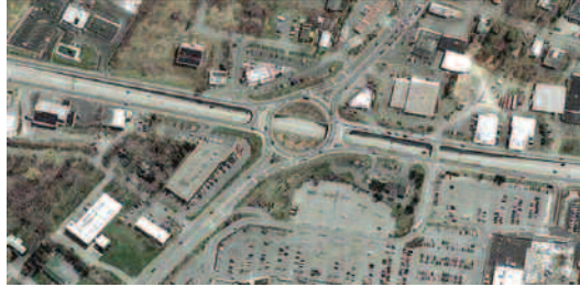
An example of continuous flow, grade-separated intersections.
