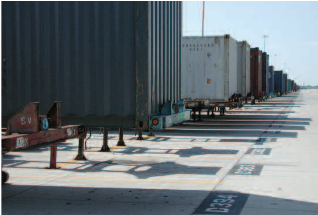
Containers often arrive at an intermodal facility by train and are then placed on trucks to be driven to the customer. These parked containers will be loaded onto truck chassis.
