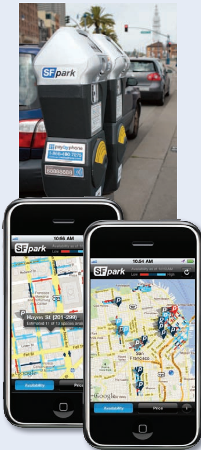
San Francisco's SFpark parking management system uses sensors to adjust meter prices based on demand. Users can access information with smartphones. (Photo courtesy SFpark)
